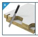
Cut or saw the service penetrations from the Multimastic FB firestop board.
